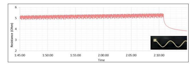
The last 25 minutes of a more than 2 hours non-stop elongation by 10%. The oscillation in the resistance and the definite decay at the end of the test should be noted. In the black box, an example of an examined track is sown.
